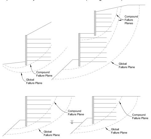
Figure 11-19: Global and Compound Failure Planes
