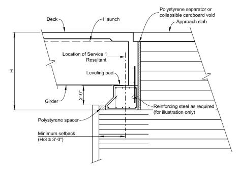
Figure 11-9: Integrated Girder Seat with Footer
