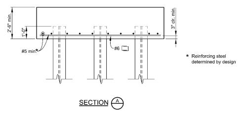
Figure 11-14: Footing on Pile
