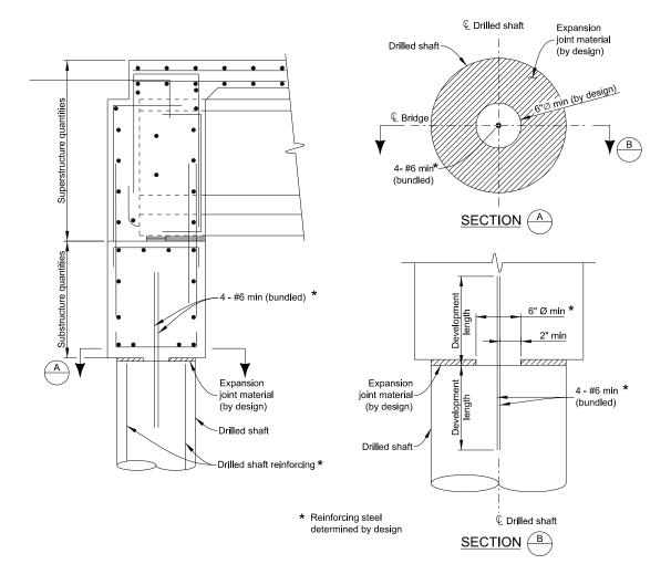
Figure 11-2: Integral Abutment on Drilled Shafts
