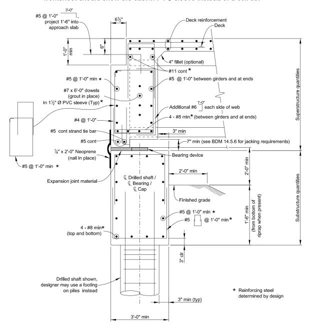
Figure 11-4: Semi-Integral Abutment (Alternative 2)
