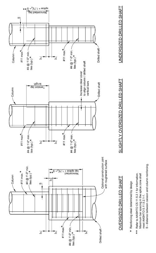
Figure 11-13: Column-Drilled Shaft Connection Details
