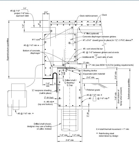
Figure 11-3: Semi-Integral Abutment (Alternative 1)
