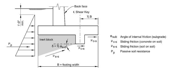
Figure 11-15: Shear Key
