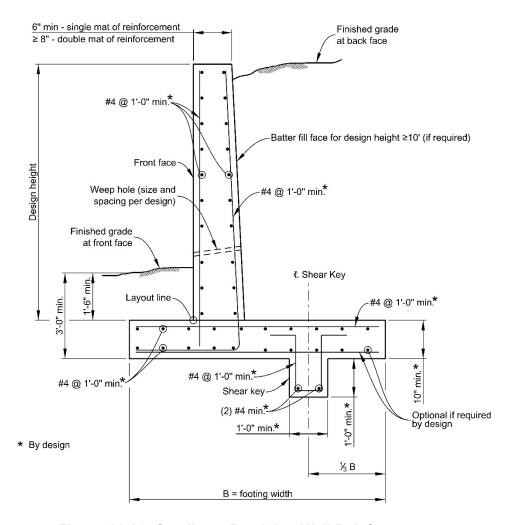
Figure 11-16: Cantilever Retaining Wall Reinforcement
