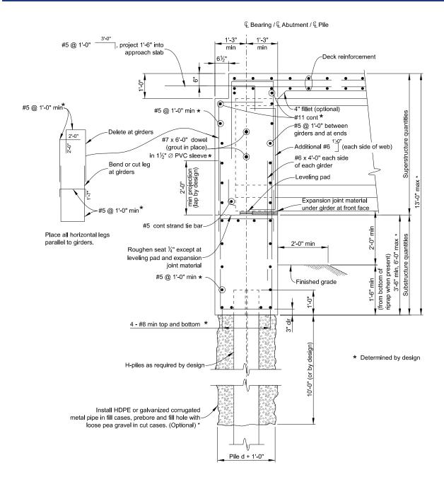
Figure 11-1: Integral Abutment on H-Piles
