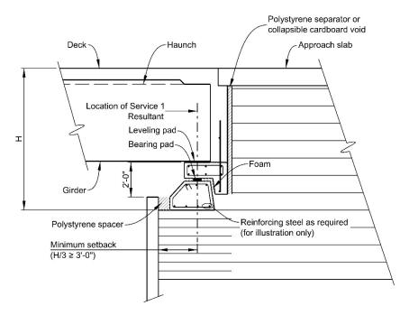
Figure 11-10: Separated Girder Seat with Footer
